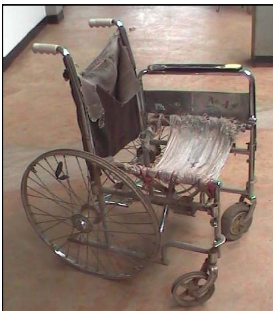
When the tyres, wheels and upholstery break on a donated wheelchair it can be difficult or impossible to repair them.
